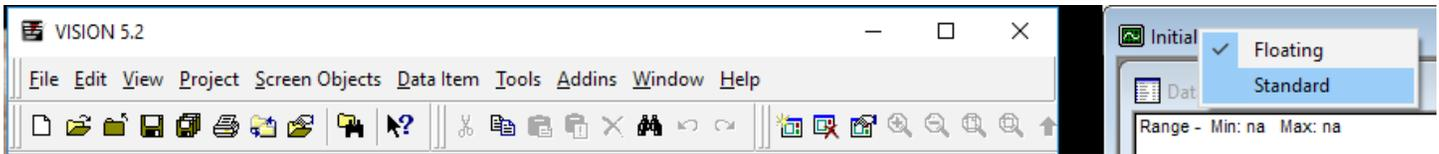
Any 'floating' window will retain its position upon closing & re-opening VISION. Additionally, any 'floating' window is compatible with touch-screens.
