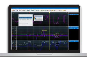
VISION Calibration and Data Acquisition Software is capable of exporting and recording directly into MDF4 format. Opening .REC files in VDA automatically converts them to MDF files and allows the viewing of recorded data that would normally have been too large for viewing within VISION. The methodology of VDA 3.0 provides users the ability to view and analyze data sets that would not be possible in a 32-bit application.
