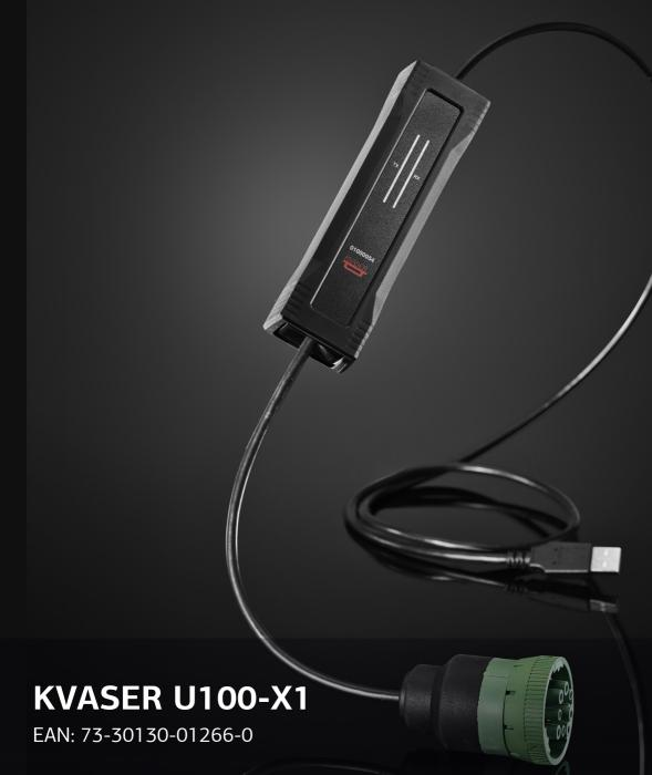
The Kvaser U100-X1 is a robust, single-channel CAN/CAN FD to USB interface with reinforced galvanic isolation that squarely addresses the needs of the evolving automotive development market. Fully compatible with J1939, CANopen, NMEA 2000<sup>®</sup> and DeviceNet, this is the first in a new range of interfaces that is also suited to rugged applications in marine, industrial, heavy duty vehicle and heavy industries.
