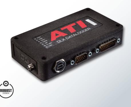
The DLX Datalogger offers a unique combination of functions that provide the features of a CAN interface, data acquisition module, and data logger all in one compact package. Communication channels include CAN and K-line that interface to ECUs or communicate with ATI data acquisition hardware.
