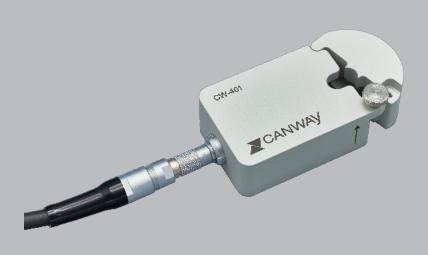
CW-401 MkII is a high-precision current clamp meter for contactless current measurement in the measuring ranges  $\pm 10 \text{ A}, \pm 30 \text{ A}, \pm 50 \text{ A}$  and  $\pm 150 \text{ A}$ . The high-quality and robust aluminium case - with very small dimensions - makes it ideal suited for measurements in rugged environments and hardto-reach places, e.g. in the engine compartment.
