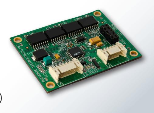
A7 Modules are a family of USB devices that provide connectivity between a PC and an Electronic Control Unit (ECU). The A7 enables data acquisition, calibration, and flashing functionality to ECUs with supported microprocessors via a connection through the microprocessors debugger interface. Currently supported interfaces include JTAG, AUD, and RTD interfaces that provide Real-Time access to memory mapped resources.
