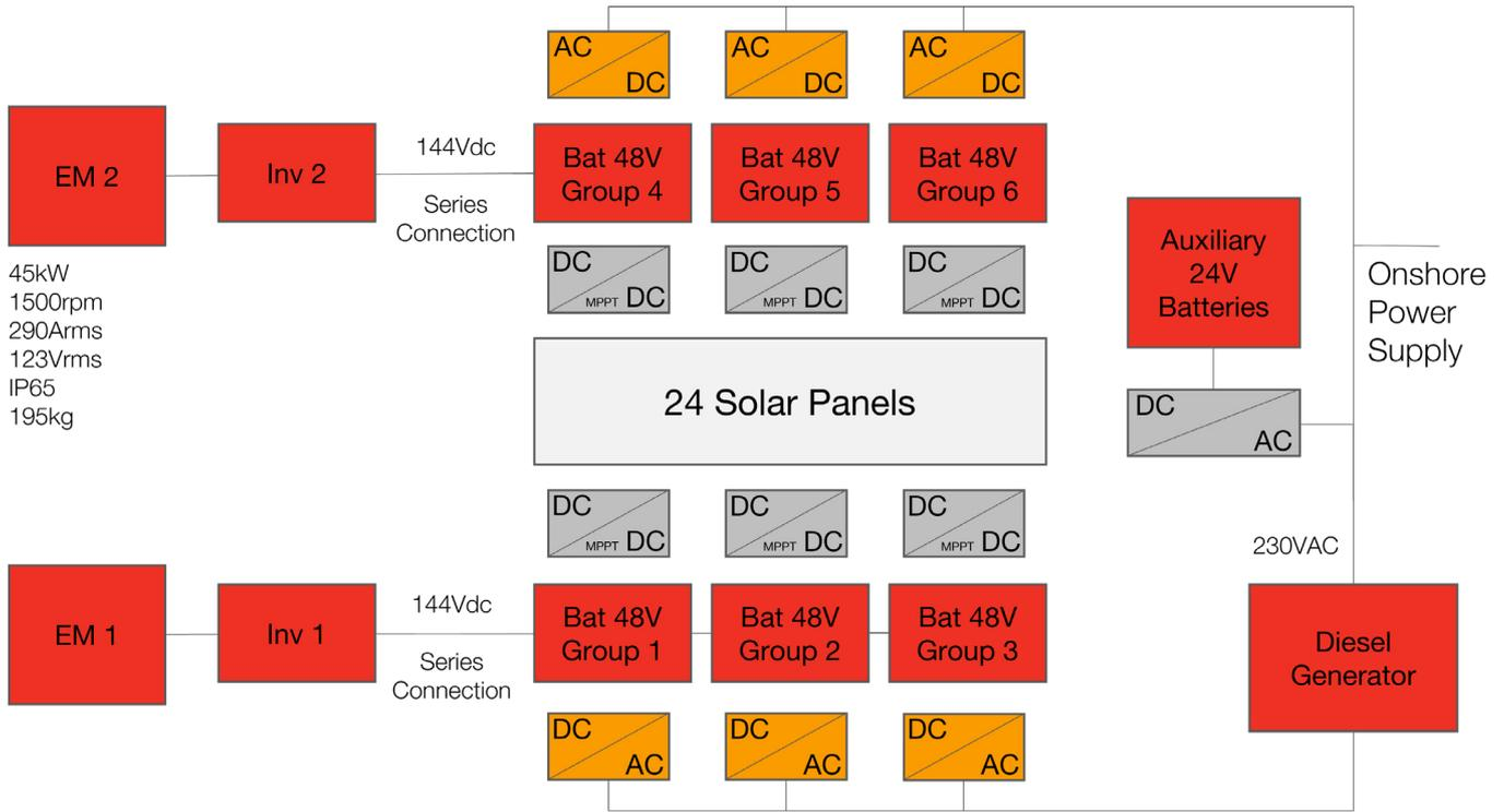
The powertrain is supplied by high voltage batteries, charged via 24 solar panels located in the roof of the vessel. In addition, a diesel generator supplies the boat's low voltage system and recharges the drivetrain batteries as a back-up power source.
